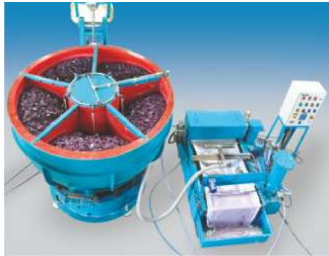
Water Recirculation System for Auto Components
