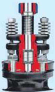
Live Loading of Valve Stem Packing Glands
