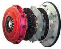
Disc spring: Dual clutch
