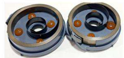
Spiral spring: Retractor spring for safety belt
